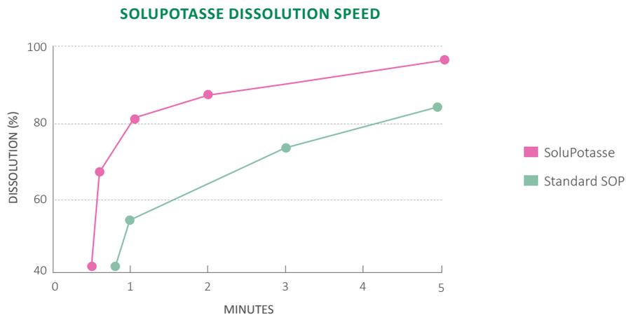
At 25°C (77°F), it normally only takes a few minutes for SoluPotasse to dissolve at a concentration of 100 g/l, which is the highest recommended practical dose. Continuous stirring and the use of warm water will speed up dissolution of the product.
